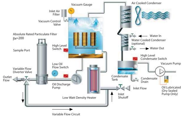
The water removal principle used in the Vacuum Dehydrators dependably removes water well below the oil saturation point, even when tightly bound in an emulsion. A vacuum pump draws fluid into the unit where it is heated and then flows through dispersal filters inside the vacuum tower. Contaminated oil flows through the pores of these filters, is exposed to the vacuum and dehydrated. Dried oil is removed, filtered and pumped back into the reservoir.
