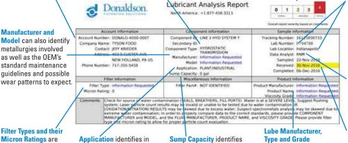
The laboratory at which testing was completed is denoted by an I for Indianapolis and an H for Houston. The following Lab # is assigned to the sample upon entry for processing and should be the reference number used when notifying the lab with questions or concerns.
